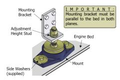
NOTE: Flats machined in top of stud to allow the stud to be held in place with a spanner while the nyloc nut is adjusted for the correct height, and for the final tightening of the top nut.
