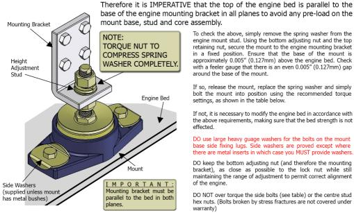
NOTE: Flats machined in top of stud to allow the stud to be held in place with a spanner while the nyloc nut is adjusted for the correct height, and for the final tightening of the top nut.
