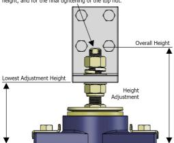
To check the above, simply remove the spring washer from the engine mount stud. Using the bottom adjusting nut and the top retaining nut, secure the mount to the engine mounting bracket in a fixed position. Ensure that the base of the mount is approximately 0.005" (0.127mm) above the engine bed. Check with a feeler gauge that there is an even 0.005" (0.127mm) gap around the base of the mount
