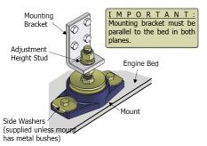
NOTE: Flats machined in top of stud to allow the stud to be held in place with a spanner while the nyloc nut is adjusted for the correct height, and for the final tightening of the top nut.
